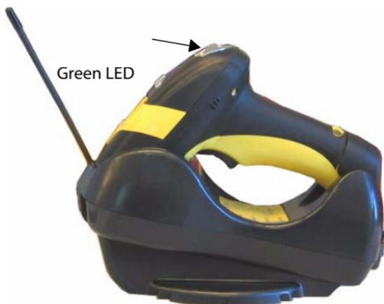
If it ever becomes necessary to change the reader, just read the bind-address label applied to the cradle and position the new reader onto the cradle.
