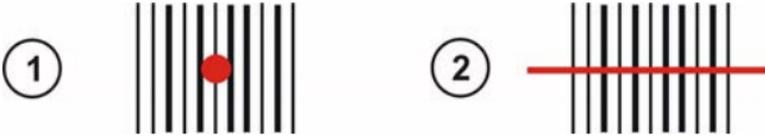
PowerScan® M8300 provides an aiming system. If enabled, a partial trigger press produces a red spot, which should be aimed over the code center to get the best reading performance, see figure (1) above. By completely pressing the trigger the scan line appears to start the code scanning (2).
