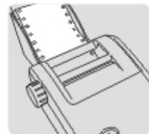
B. Turn the paper loading knob in the clockwise direction. Until the paper is suitable.
