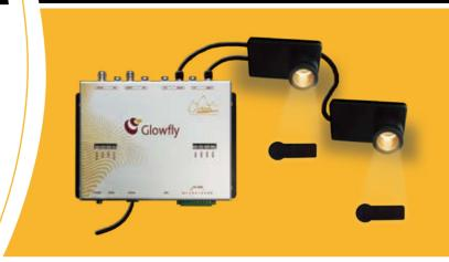
• Target selective characteristics with visible LED lights. Just one wanted tag or tag groups can be read using LED beam.
